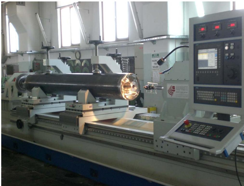
The tooling which can be used on this machine are BTA or STS type.
