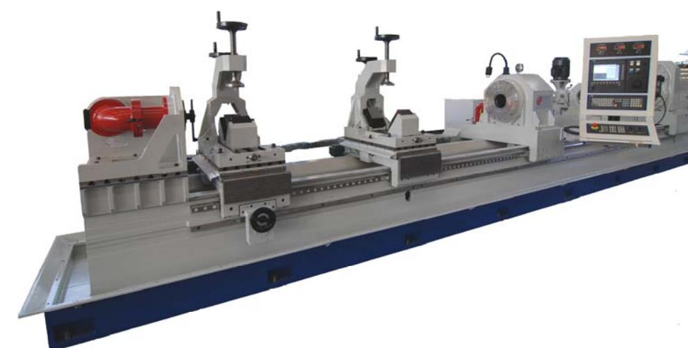
With today's technology in drilling and pull boring, counter rotating machines are no longer needed. The machine works on the principal of a clamped workpiece and rotary tools thus allowing the drilling and boring of non rotosymmetrical workpieces as in twin-screw barrels.
