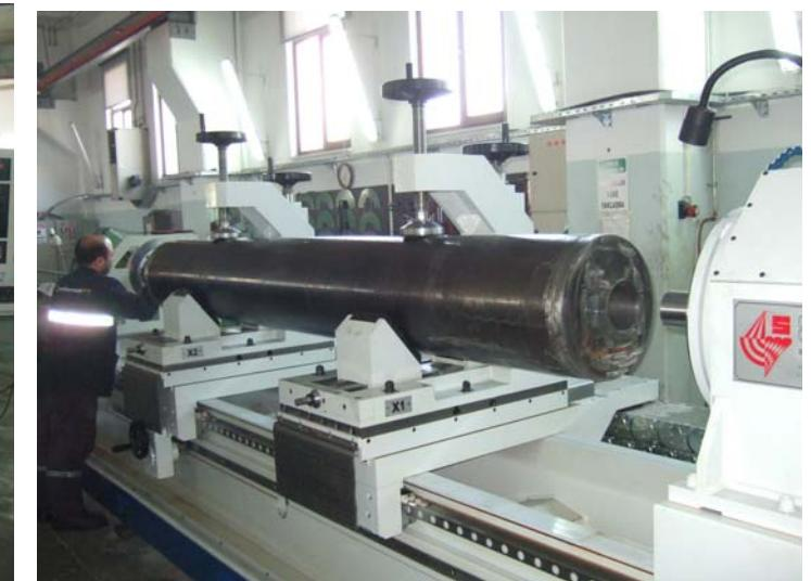
There are six controlled axis, four linear, Z1 longitudinal length of the machine, Z2 longitudinal of steady rest (lapping head optional), X1 transversal first carriage, X2 transversal second carriage and one rotary, S1 rotation drilling tool.
