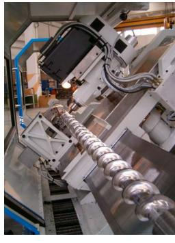
The bed is in electrowelded steel structure stress relieved with grinding surfaces to hold high precision guideways for rollers sliders.
