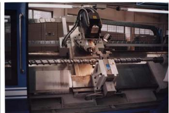
The machines are equipped with CNC, motors and drivers Siemens. The milling head motor power is 22 Kw. The spindle nose is ISO 50. Max spindle speed 5000 rpm.
