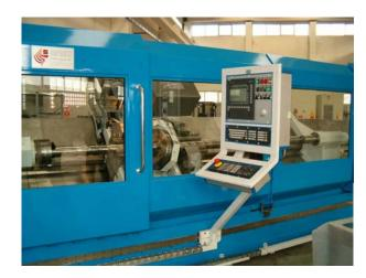
Our threader machines are equipped with CNC Siemens of latest generation (840D) and can be optionally equipped by Renishaw tool probe and tool changer
