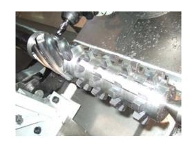
Our models GRM have whirling head and are suitable for big series of screws
