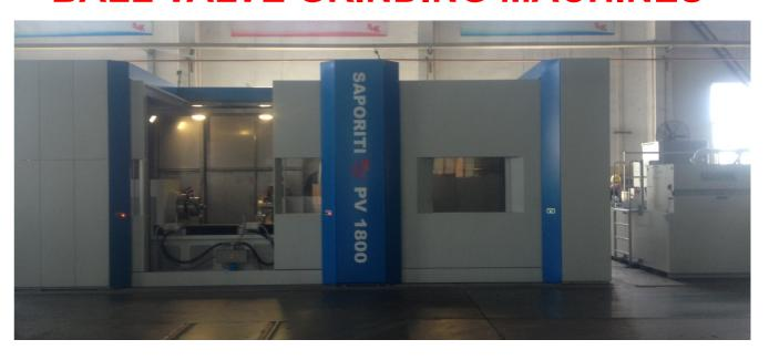
The new generation of valves balls are manufactured especially for metal to metal seats valves and are often coated by extremely hard materials. The ball valves grinding machines series **SAPORITI PV** are available in different sizes to work balls **from 1" up to 64".** These machines are the latest results of a very long experience to assure a reliable and accurate production to our Customers. The roundness precision which can be achieved can satisfy more even the most demanding customers
