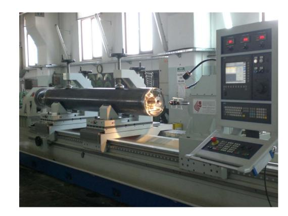
The tooling which can be used on this machine are BTA or STS type.
