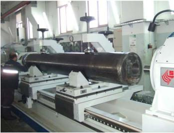
There are six controlled axis, four linear, Z1 longitudinal length of the machine, Z2 longitudinal of steady rest (lapping head optional), X1 transversal first carriage, X2 transversal second carriage and one rotary, S1 rotation drilling tool.
