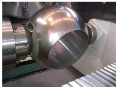
Also the second valve was finished with an accuracy of: Less than 0.01mm roundness
