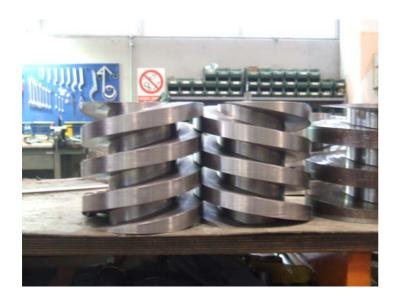
The machines rigidity allows for high chip removal and very good surface finishing. It is possible work up to 80 mm depth by only one passage.
