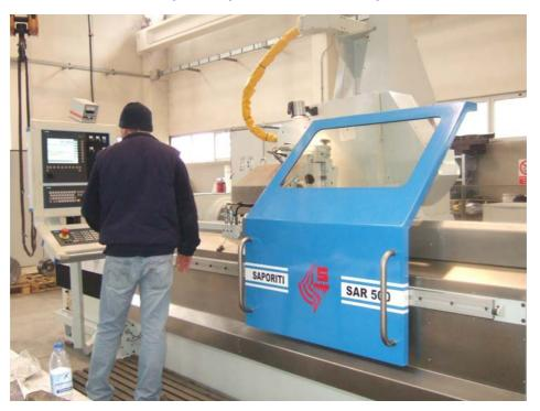
The New **SAPORITI SAR** is a CNC machine for the manufacturing of pump or compressor screws by Disc Cutters.
